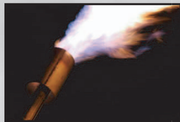
Landfill gas will be used to power the engine/generator instead of being destroyed at the flare
